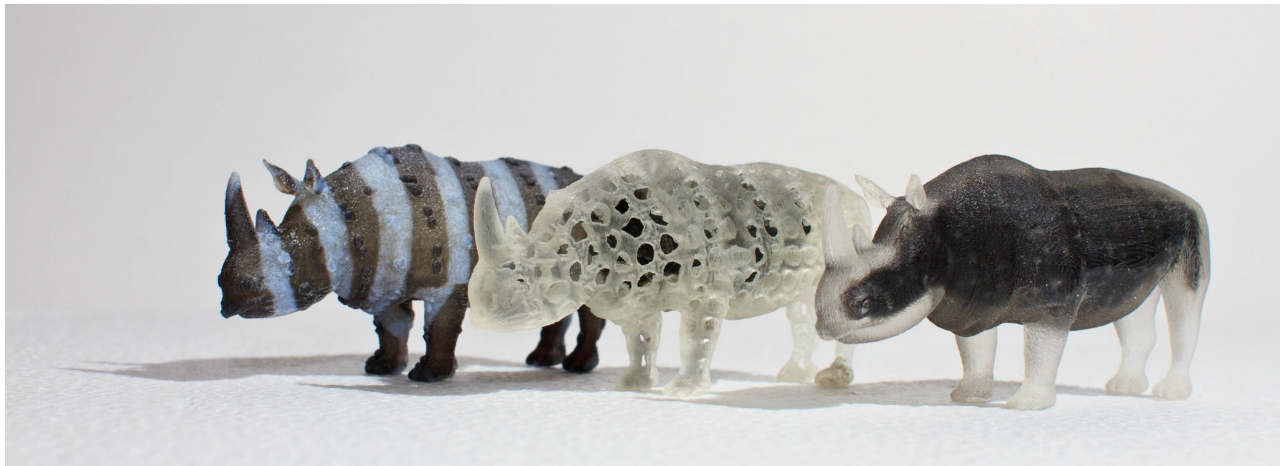
Figure 1: Three rhinos, defined and printed using OpenFab. For each print, the same geometry was paired with a different fablet—a shader-like program which procedurally defines surface detail and material composition throughout the object volume. This produces three unique prints by using displacements, texture mapping, and continuous volumetric material variation as a function of distance from the surface.
